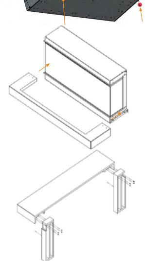
**15)** Screw the two legs of the surround from the rear onto the back of the top section of the surround as shown.
