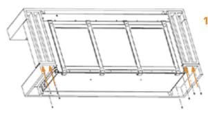
17) Underneath the appliance, with the surround screws, screw up through the bottom surround and into the legs of the surround top section and up through the floating shelf brackets on the appliance and the top section.
