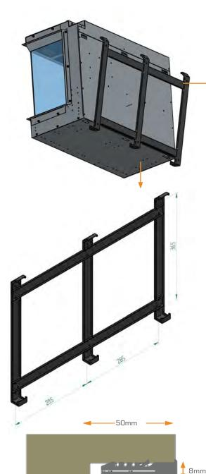
Before Installing the appliance onto the wall with the suite, secure the side trims each side of the appliance as described in section 8.0 Preparing the Appliance.
