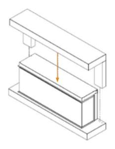
**16)** Carefully lower the top section of the surround onto the top of the firebox.
