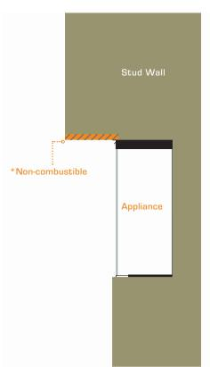
\*If the stud wall immediately above the heater protrudes beyond the front of the appliance then the over-hanging section of the installation must be made from a non-combustible material, such as calcium silicate fireboard.
